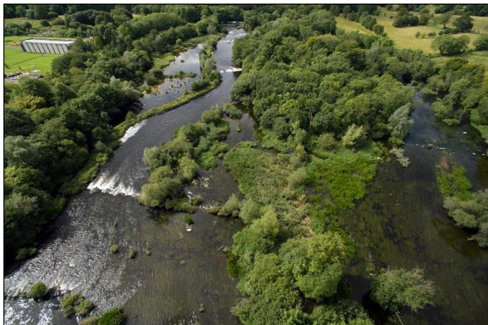
Plate 4 Extreme water abstraction / regulation has had a profound impact on the old River Shannon within the study area. Flows are generally only 10 cumecs (which approximates the n99%ile flow).
