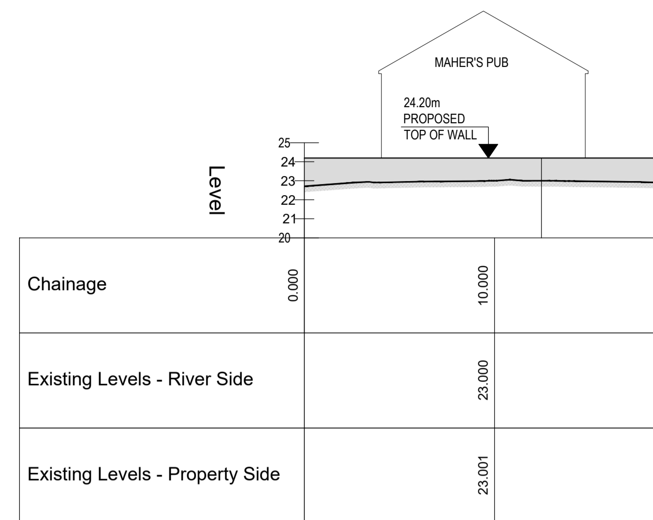
WALL 5B - LONGSECTION SCALE: H 1:200, V 1:200. DATUM: 20.000 WALL 5B LONGSECTION SCALE H 1:200, V 1:200
