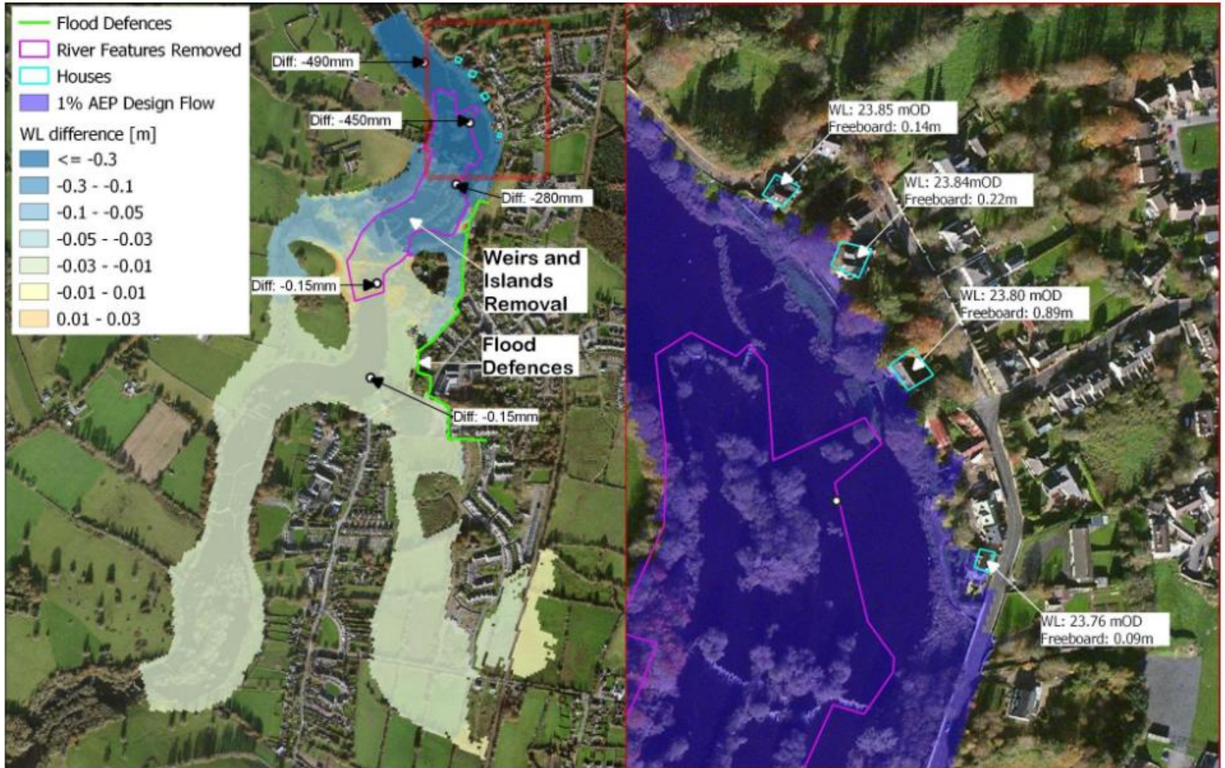
Weirs and Islands Removal Walls Downstream of The Elvers Rd
